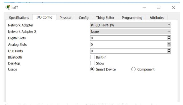
Change the **Network Adapter** drop down list to **PT-IOT-NM-1W**, which is a wireless adapter.
