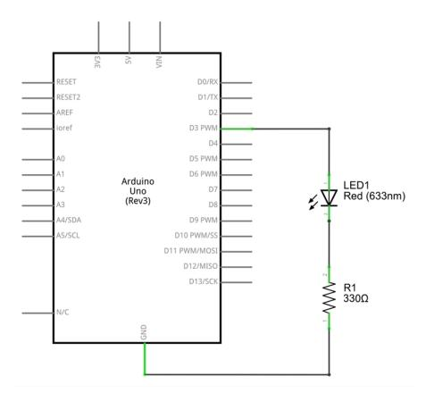
The LED has two legs: one is called anode, while other one is called cathode. To light up the LED, charge the anode to about +2V and the cathode to the Ground (0V). The anode leg is generally longer than the cathode leg but it is not a standard. On the other hand, the cathode leg is always connected to the bigger part inside the LED.
