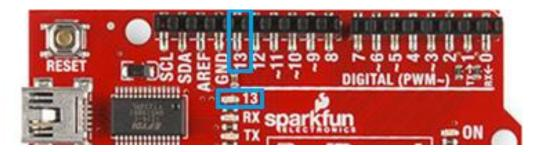
c. Predict the output of the **loop** function. The **digitalWrite** function sets the value of pin 13 to HIGH. A **delay** function will then pause the execution for 1000ms. The next use of the **digitalWrite** function will set pin 13 to LOW, followed by another delay of 1000ms. Upon completion the **loop** function executes again. The loop will repeat until the RedBoard is turned off:
