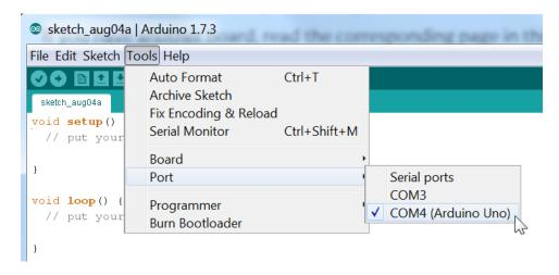
**Note**: Linux users will find that the Arduino IDE requires the addition of dialout group access to use /dev/ttyUSB0. For a genuine Arduino UNO board, the actual port that is used is /dev/ttyACM0. The number 0 identifies the first connected board. Additional USB connected boards will be identified with respective numbers such as 1, 2, 3, etc.
