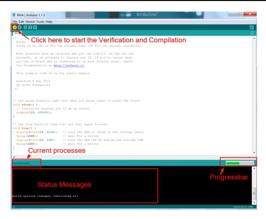
e. Upload the firmware to your RedBoard. After this step, you should see the onboard **LED** connected to pin 13 blinking in a 1 second interval.
